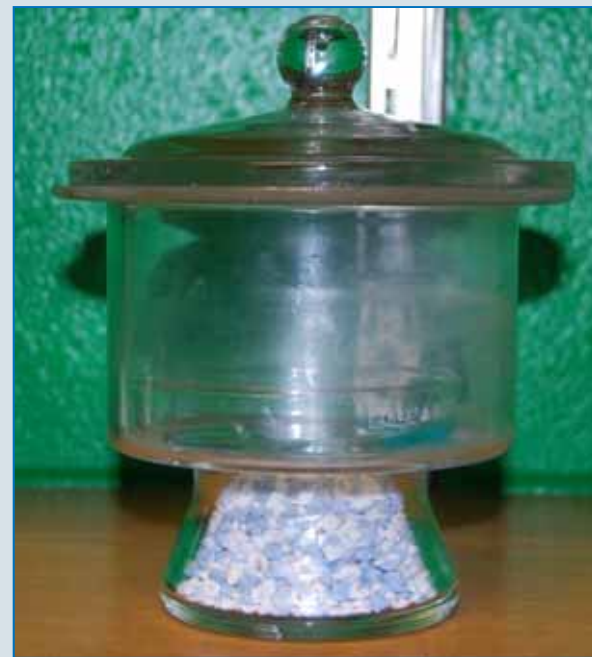
Inside a desiccator with desiccant, some use a vacuum desiccator.
